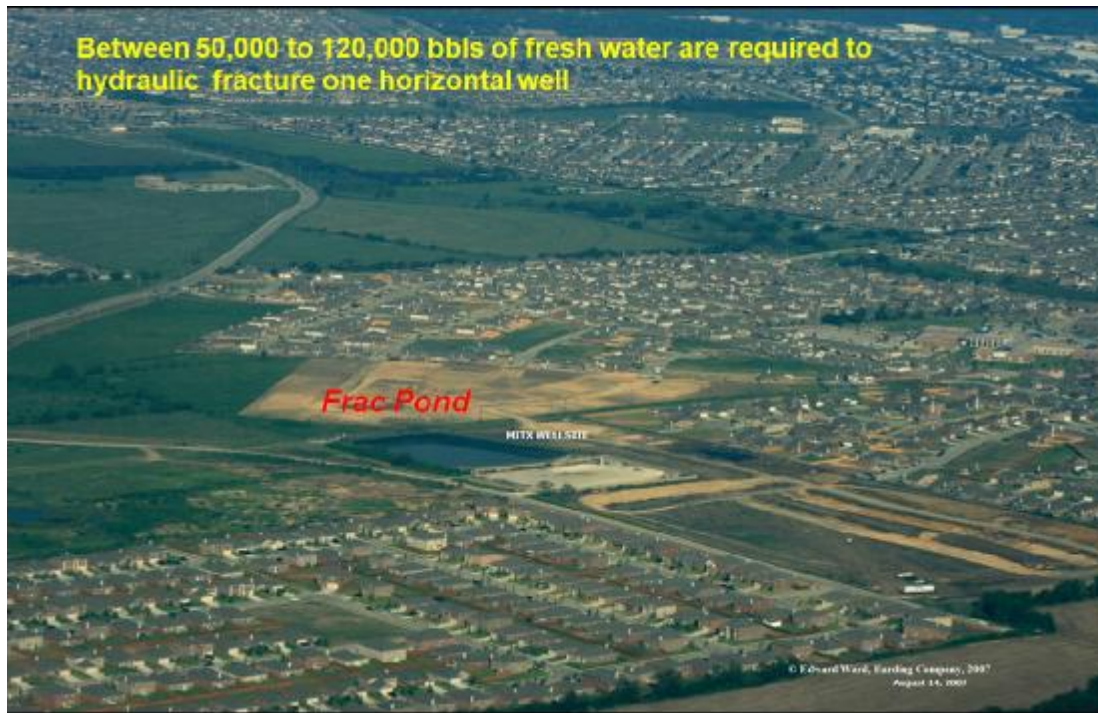
Urban well site with fracture water pit, Barnett shale, Tarrant County (Harding-ExxonMobil, 2007).
