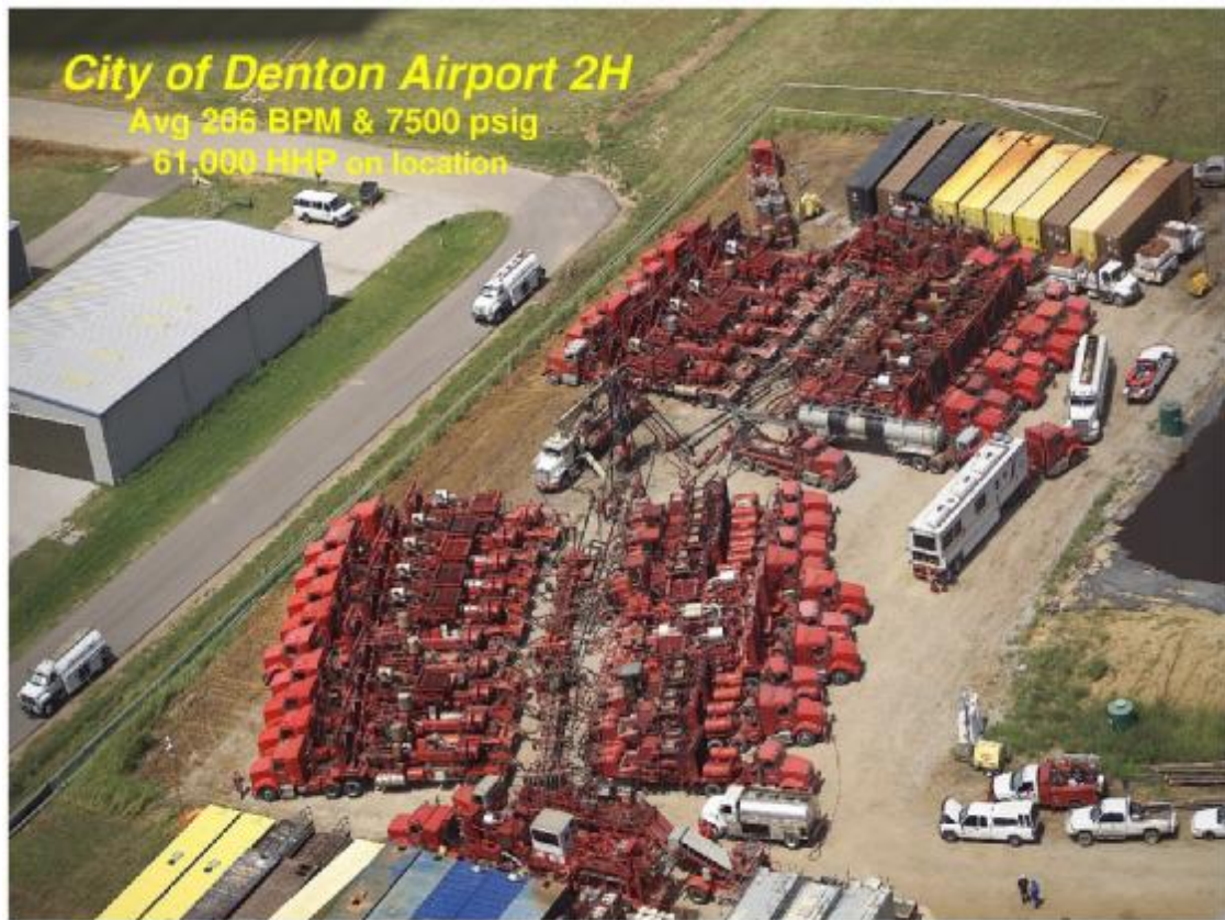
Hydraulic fracture, Barnett Shale, Denton County Airport. This is an example of logistics of an older well completion technology and engineering techniques. Better understanding of rock mechanics and more efficient pumping equipment have greatly reduced the amount of equipment required (Matthews, 2004).
